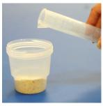
Add 3 mL/g of distilled, deionized, or bottled water (eg: 150 mL for 50g sample)
