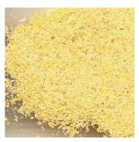
Collect and grind a representative sample such that ≥95% passes through a 20 mesh sieve
