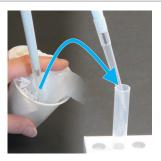
7. Transfer 100  $\mu$ L of the clarified extract to the tube; stir well with pipette tip
