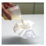
Filter extract using approved coffee filter into a clean vessel
